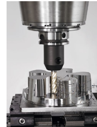
Solid carbide milling cutter MD133 Supreme from Walter Prototyp in use.
