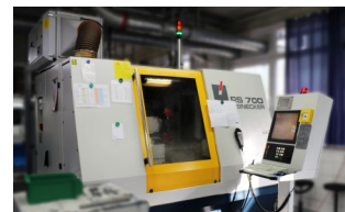
Tool grinding machines with NUMROTO software in ALMÜ's machine park
