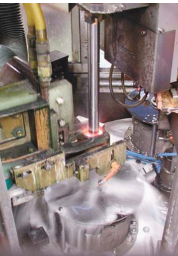
Inductor movement relative to the part must be flawlessly controlled.
