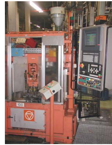
Retrofitted with an Axiom Power, this induction quenching machine is used for processing steering rack shafts.
