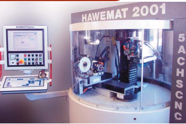
The Hawemat 2001 CNC grinding machine is the most sophisticated of the Hawema 5-axis grinding machines equipped with a CNC.
