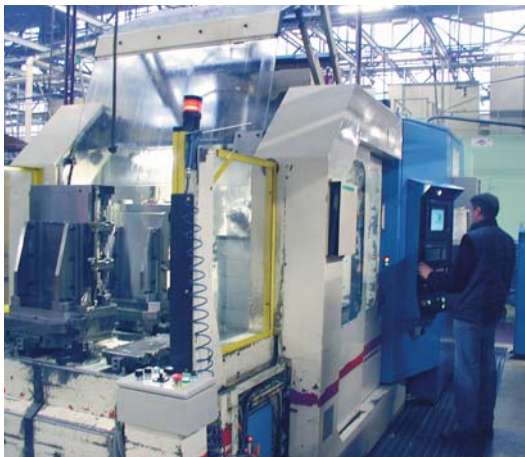
This retrofit was especially beneficial by making the tool changer control more reliable and optimizing it.
