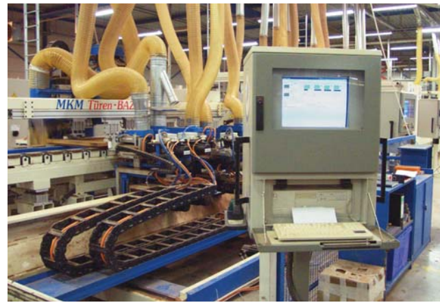
Five Num 1080 CNCs control the system machining stations. They are integrated in a TCP/IP network and communicate with a special server program.
