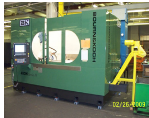
Bourn & Koch's 400H Series II gear hobber has seven CNC axes
