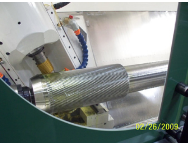
The 400H gear hobber features a unique CNC servo-driven tailstock
