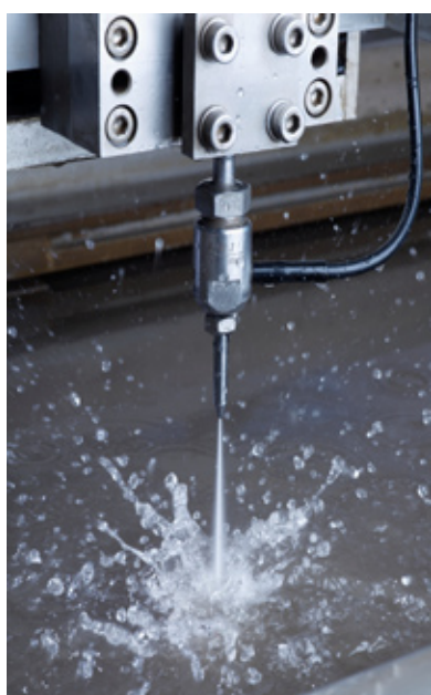
highly precise water jet >0.3mm
