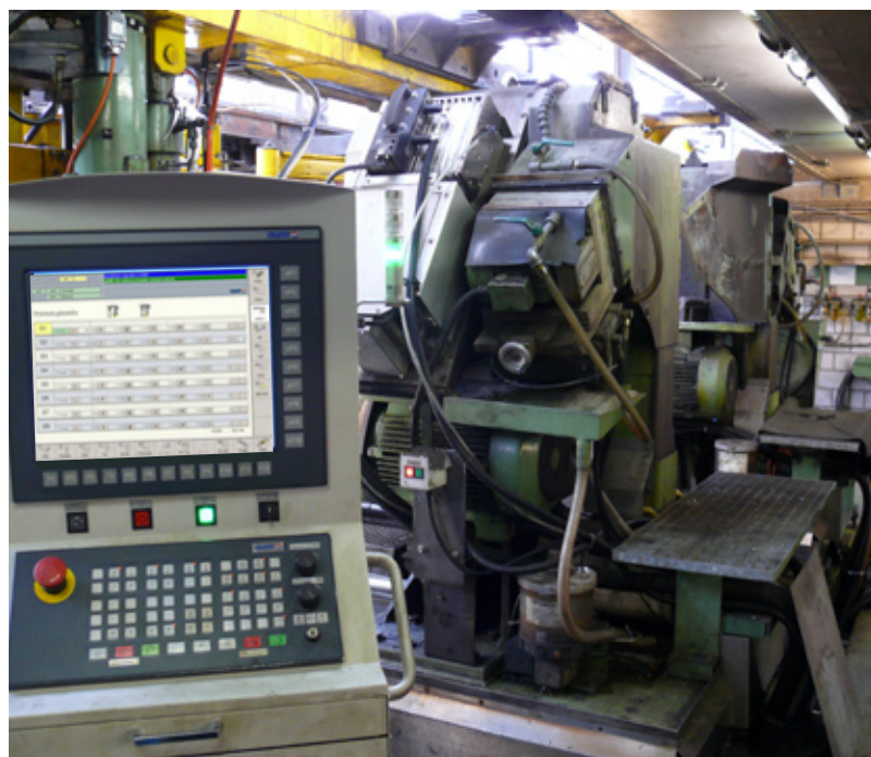
Control panel for underfloor wheel grinding machine
