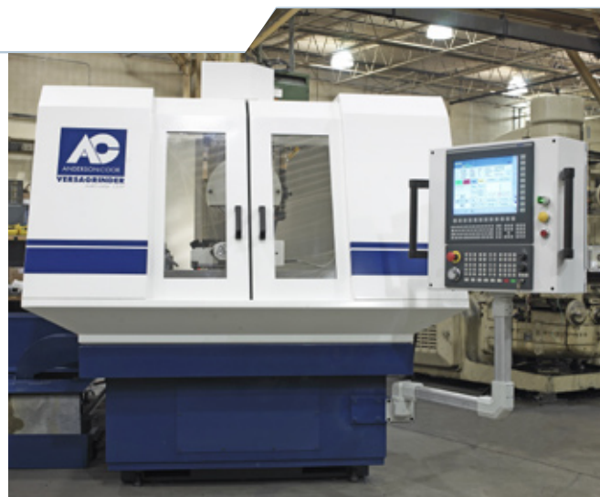
Anderson-Cook's new AC-Tru Grinder tool grinding machine uses a 3-axis NUM Power CNC system
