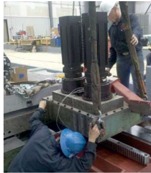
Tandem drive pinion assembly is managed by NUM MDLU3 drives
