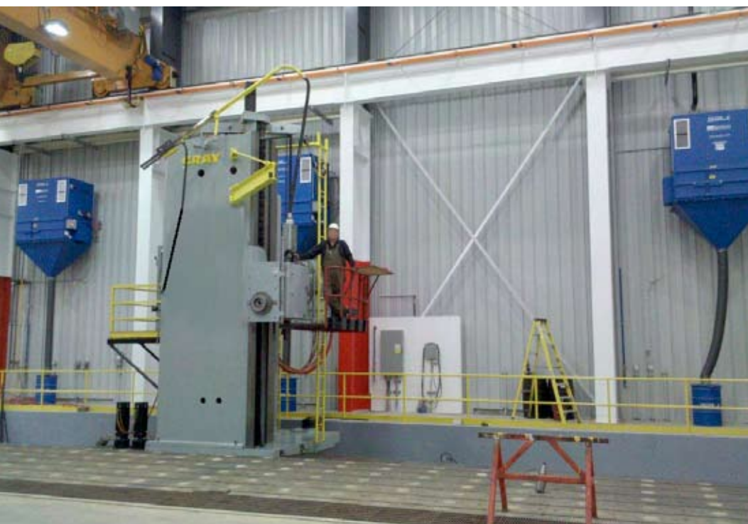
Accuracy of the large mill is ensured thru NUM's adaptive axis compensation
