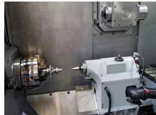
Genymab's work surface with the tailstock and the milling work table on the right
