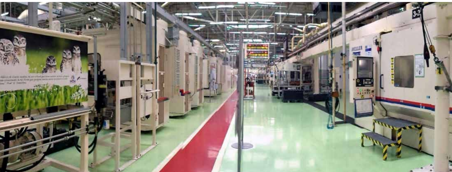
Below: The crankshaft production line at Fiat Powertrain's Campo Largo plant makes extensive use of CNC machines
