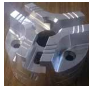
Inclined plane and RTCP processing (5 axis): Offline simulated work piece and machined part
