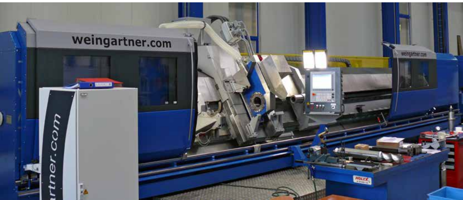
Below: Vario production machine from Weingärtner Maschinenbau GmbH with a NUM Flexium CNC system
