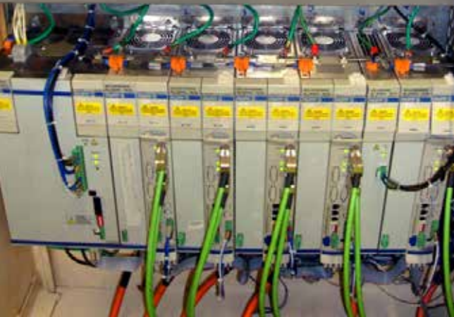
Top: Prior to the upgrade, the controllers for each CNC machine on the crankshaft production line were based on early-generation NUM 1050 series CNC
