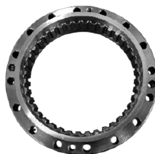
An internal gear after profile grinding.
