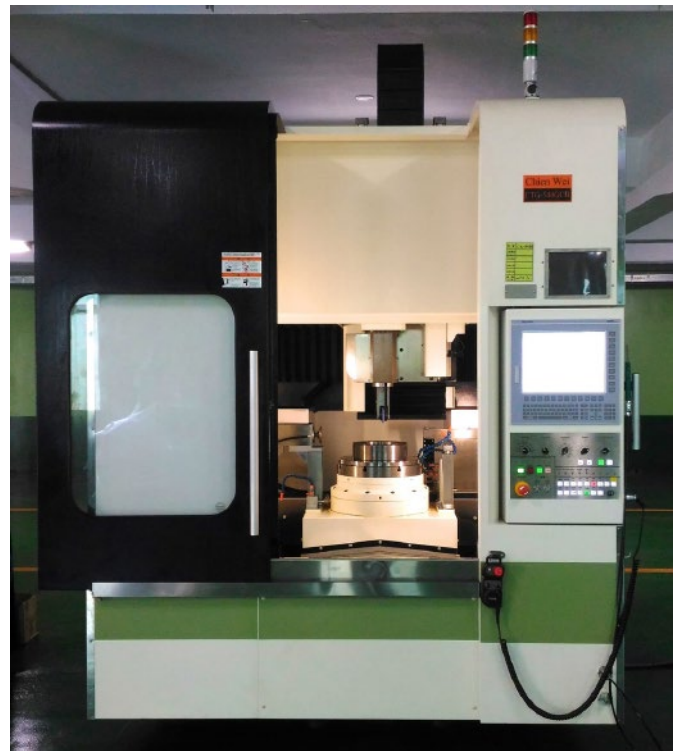
Chien Wei's new gear grinding machine is based entirely on NUM's latest-generation Flexium+ 68 CNC platform.
