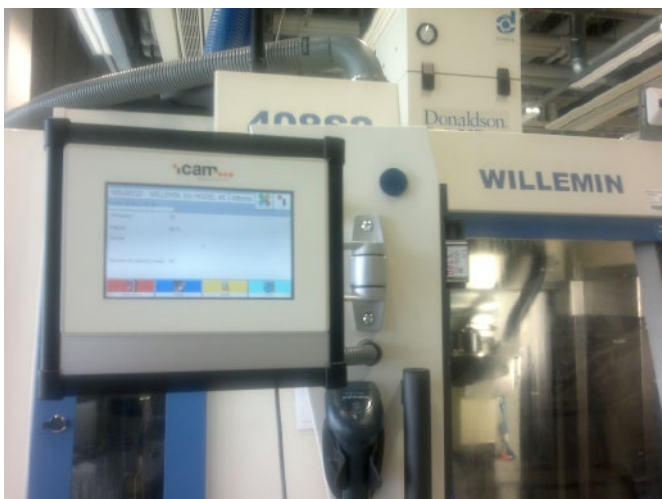
Terminal on an analog CNC machine to connect it to iCAMNet.
