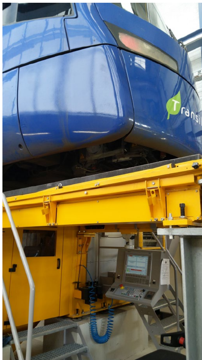
View of the operator's spot just after tramway positioning.
