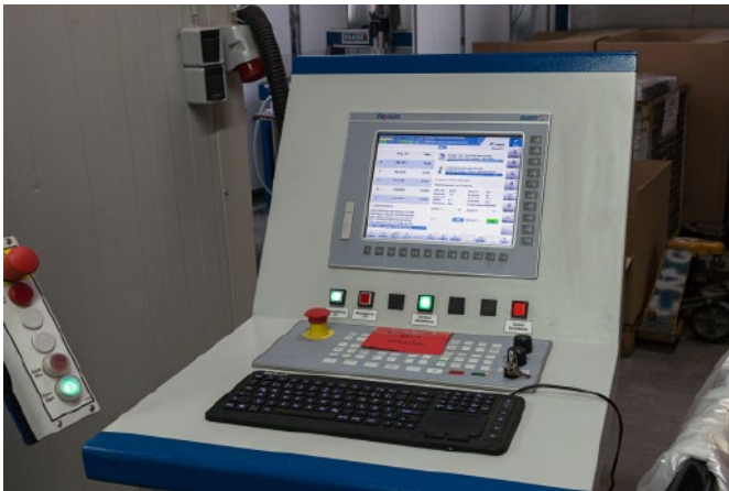
Remote control panel FS122 with machine control panel MPO4 of the NUM Flexium+ system.
