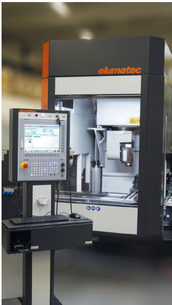
FS154i P2 control panel (with SSD and Quad-core processor) and MPO6 machine control panel from NUM.
