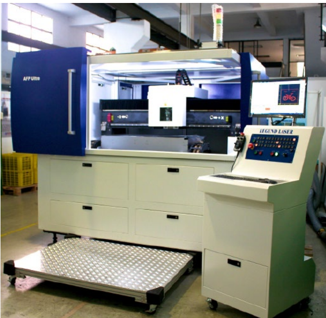
Legend Laser's new SRC-610 precision sheet metal laser cutting system is based entirely on NUM's Flexium+ CNC platform.
