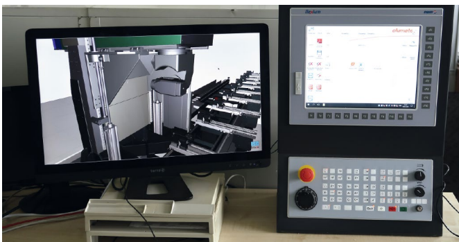
In the virtual commissioning system at elumatec, all control components are virtually reproduced one-to-one. The machining head of the SBZ 151 can be seen on the screen
