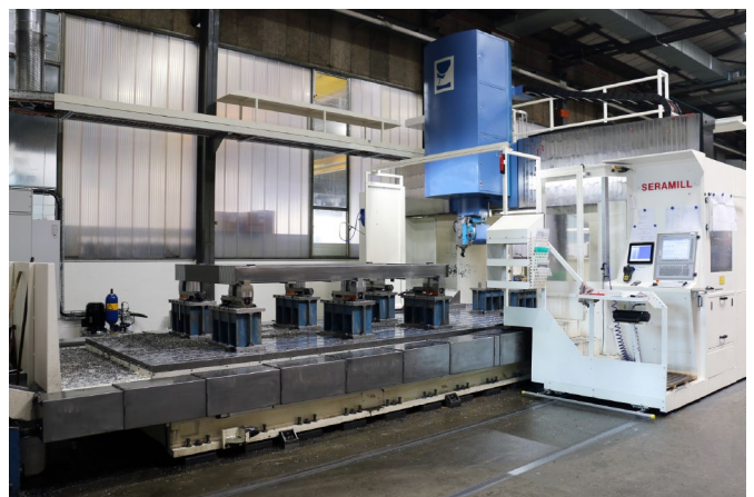
Seramill portal machining center with NUM CNC control Flexium+
