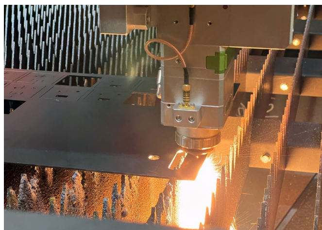
Example use of Intersample M, the laser will be interrupted between each hole and restarted immediately
