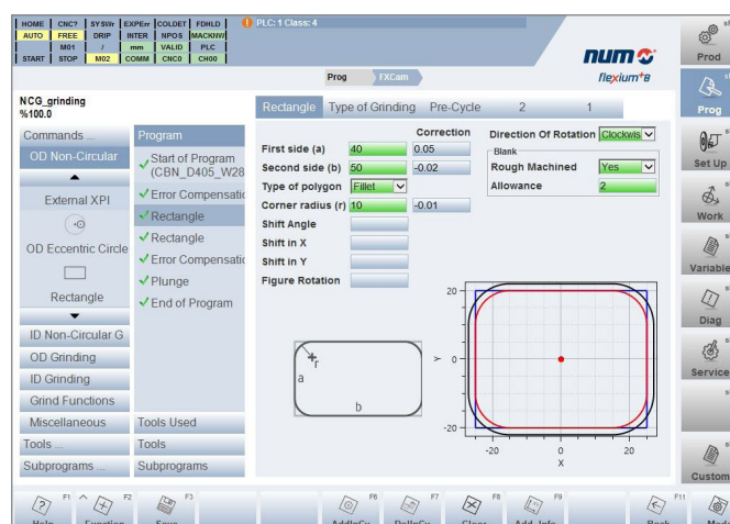
NUMgrind software helps to completely automate non-circular grinding
