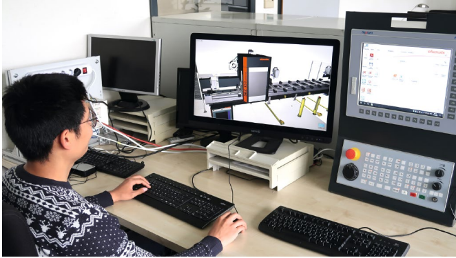
An employee simulates the functions of an SBZ 151 on the virtual commissioning system at elumatec AG
