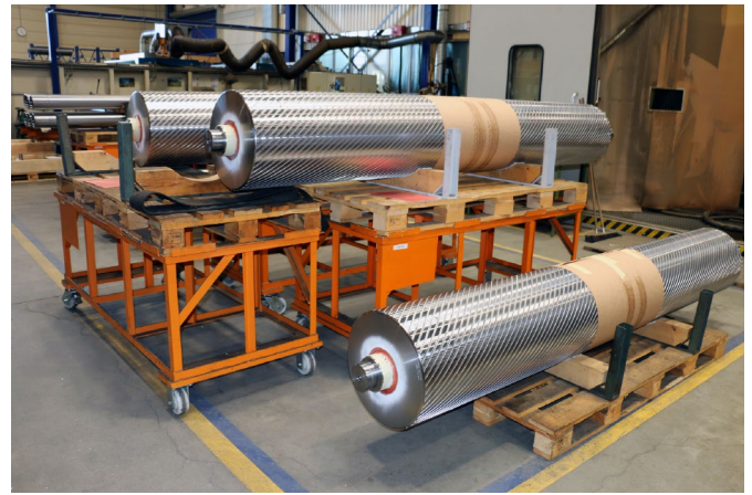
Rolls after machining by the groove milling machine
