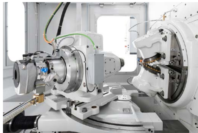
The cooperation between NUM and Lanzi has existed for a long time and has deepened over time through various projects. The most recent project is the retrofit of an old bevel gear hobbing machine for cutting straight teeth
