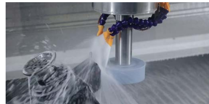
Automatic dressing of grinding wheel
