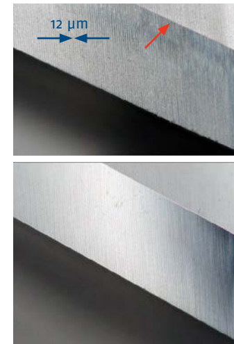
Figure 3 Image of the 1 st relief in 200x magnification, top with a non-dressed grinding wheel, bottom with a dressed grinding wheel
