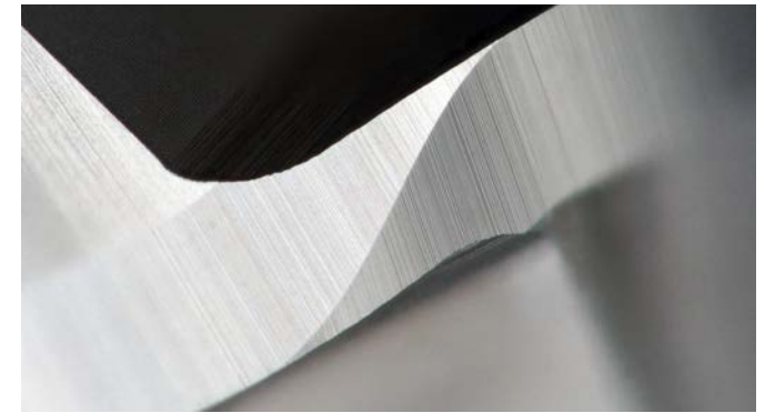
Figure 1 Transverse cutting edge measured with the Keyence digital microscope (magnification 200:1)
