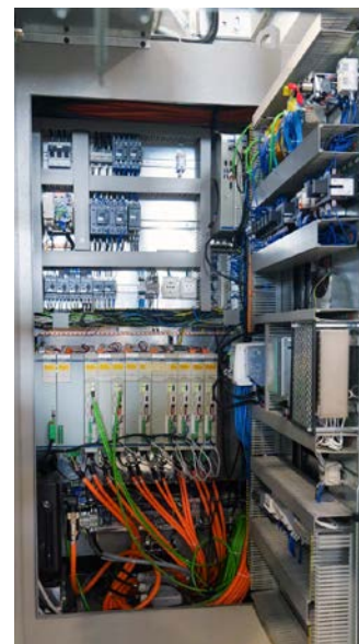
Techno Multiwall is equipped with Flexium+ 68 numerical control system supplied by NUM with motors and drives
