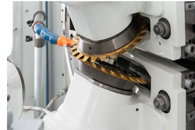
The project focused on the design of the two milling heads (originally driven by a single motor) by inserting two motors into them to achieve a higher speed
