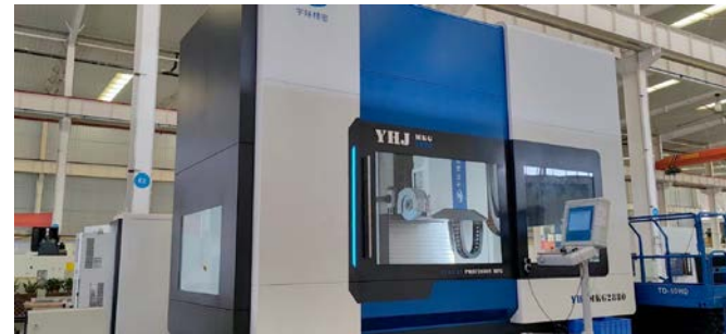
YHJMKG2880, a high precision CNC universal vertical grinding machine
