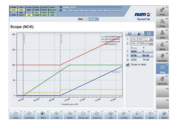
All these features are easily programmed with a single G function and a few parameters. For example, "Z100 G777 Q1 X40 P24 I25" tells the control to move the Z axes to the position Z100 mm, when 40 mm have been travelled the PLC output bit 24 will be set, and when the PLC input bit 25 is set then the execution of the next block will start, even before the Z axis has arrived at it's final position.
