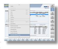
mand entry. The NUMmill HMI displays commands, grouped into specific submenus by operation type. A status icon is displayed next to the program step indicating errors/incomplete input or that data entry is complete. The first step to create a new program is to add the "General Definition" command from the "Miscellaneous" menu.
