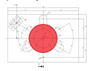
In the "Pocket Milling" menu the command "Pocket definition" offers the possibility to select three types of pockets (Circle, Oblong and Square). The user enters the correct data according to geometric and process re-
