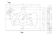
In the mechanical drawing the user identifies the required tools and determines the program origin, OP: Milling tool (trochoidal) for pocket machining (R = 3 mm) Drilling tool for the 2 mm holes (R = 1 mm) Datum set OP in the center of piece
