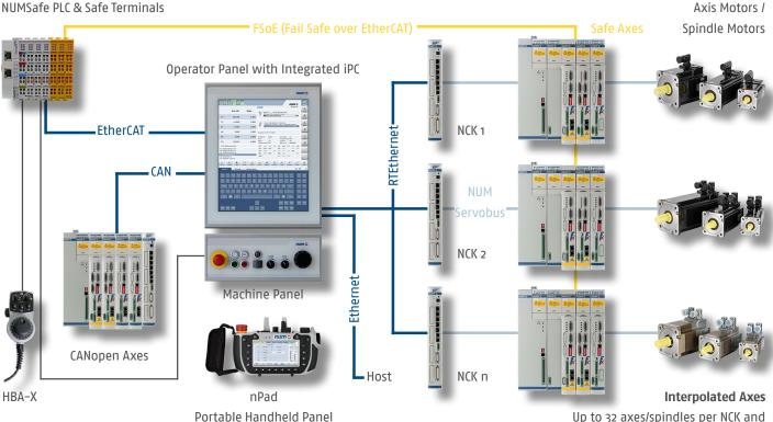
Up to 32 axes/spindles per NCK and more than 200 per CNC system
