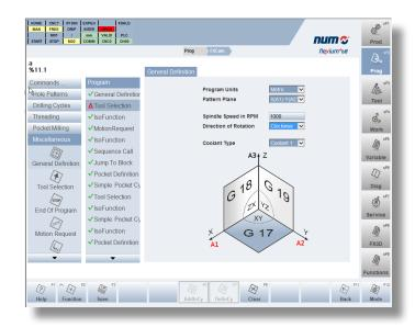
Hole patterns can be programmed in a variety of geometries, including Arc, Cover Patter, Drilling with Rotary Axis, Grid, Pitch Circle, Row, and Single Points.
