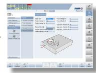
Inserting an "ISO Function" command allows for shifting or rotating the pocket's position.
