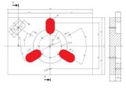
The Hole Patterns menu includes several possibilities: Arc pattern, Cover, Grid, Drilling with rotary axes, Pitch circle etc.
