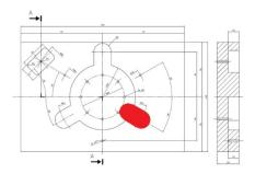
Like in the prior operation, the pocket geometry is first defined, followed by the "Simple Pocket cycle" to enter the process data
