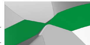
Figure 5 Simulation of a cross-gash out
