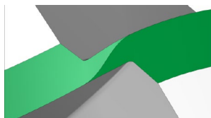
Figure 4 Simulation of an S-shaped chisel edge
