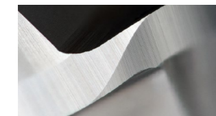
Fig. 1 Transverse cutting edge measured with the Keyence digital microscope (magnification 200:1)
