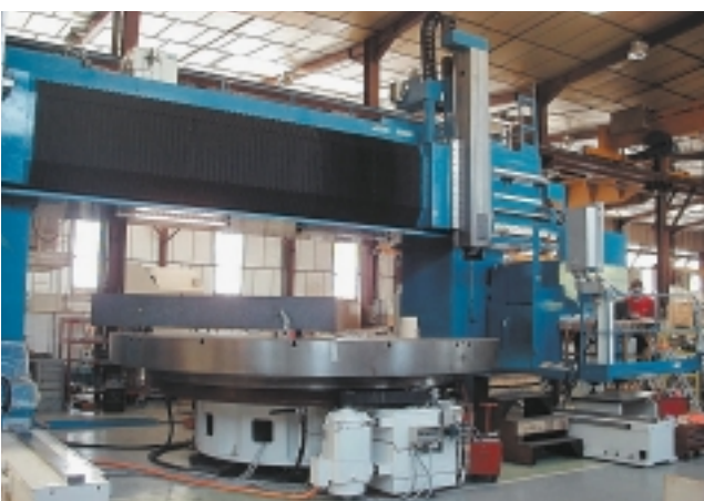
Dufieux Industrie turning-milling machine being assembled and its 4.5 m turntable.
