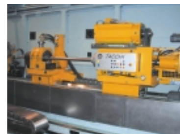
Second spindle for holding the workpiece for turning or the tool for boring
