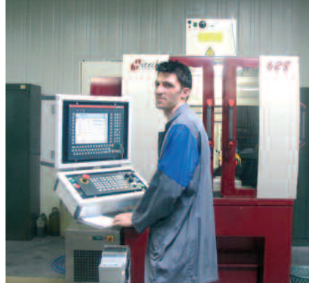
The Witech 628 machine is a 5-direction machining center that is specially suited to making very high precision parts.
