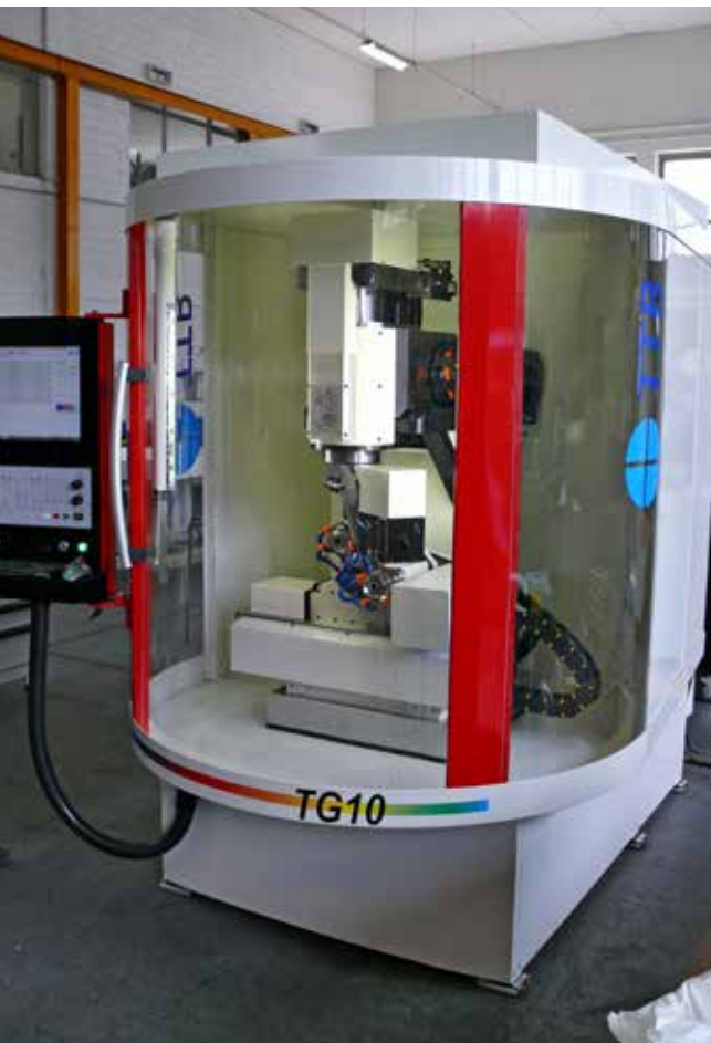
TTB TG10 high-precision grinding centre
