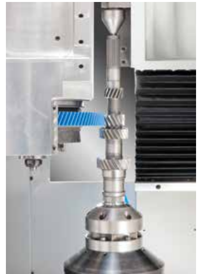
Input shaft of sports car transmission honed with GRONO 250
