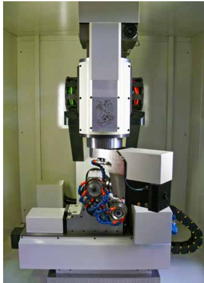
On the left: TG10 kinematics with high stability and rigidity thanks to a compact design and innovative vertical axis principle
