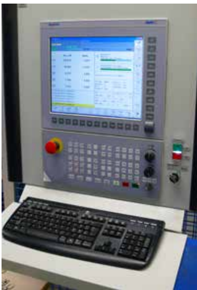
Control panel with NUM Flexium HMI
