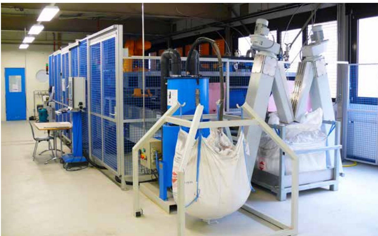
Complete water jet cutting machine, showing operator's control station and process waste disposal unit
