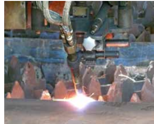
Flame cutter utilising the angle-cut function
