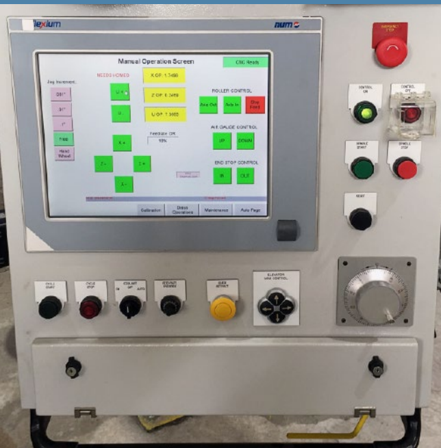
Above: The machine's new control console incorporates a Flexium operator panel with a touch-sensitive display screen.
