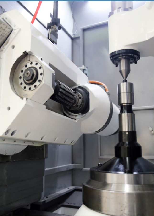
Above: Direct drive motors controlled by NUMdrive X servo drives power the turret spindle and table in Betek's new gear cutting machine.
