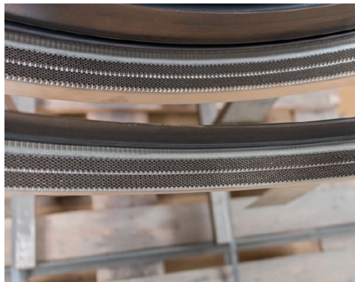
Below right: detailed picture of the ultra-fine honeycomb structure of the engine part of an aircraft turbine.
