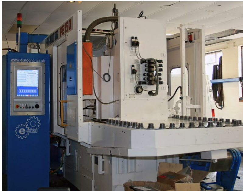
Top right: a retrofitted Pfauter PE150 gear hobber.
