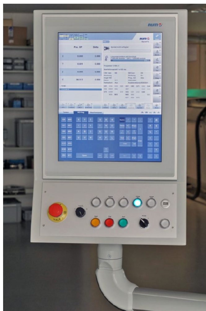
NUM FS192i HMI, complemented by the operating panel developed in-house by Felastec.
