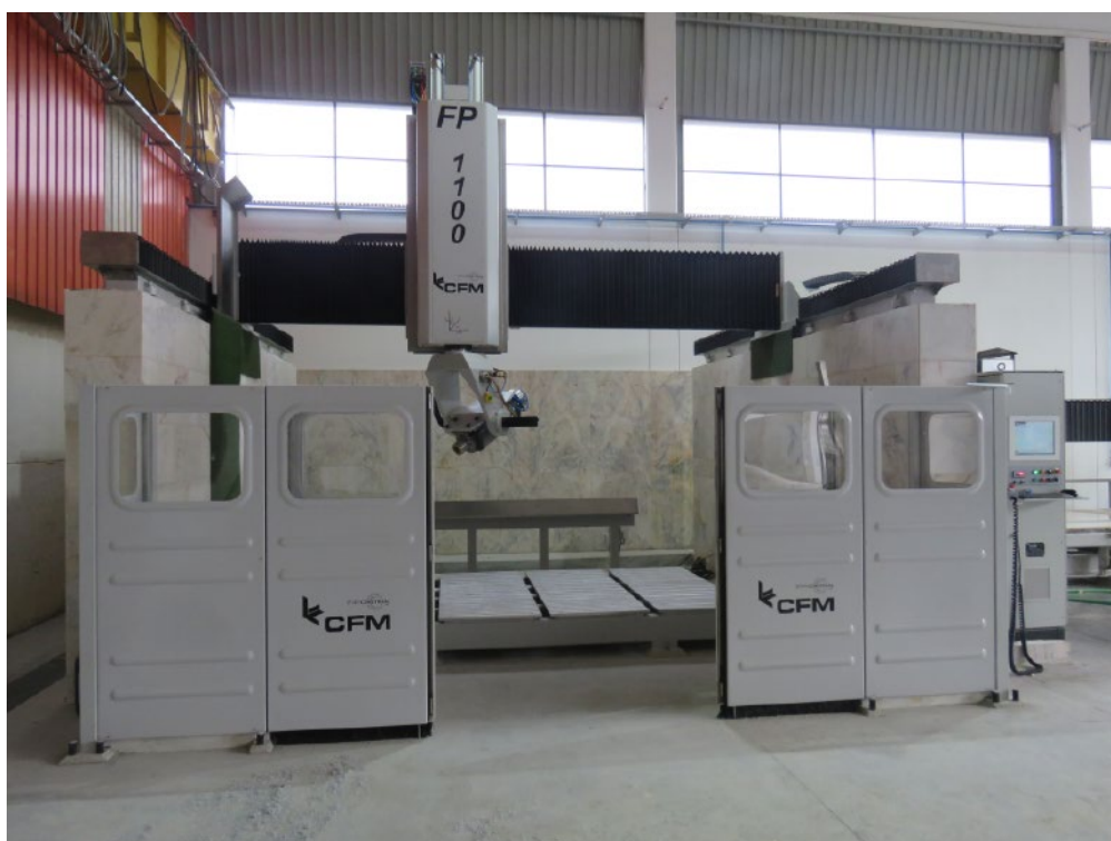
5-axis CNC gantry machine from CFM with NUM controller.
