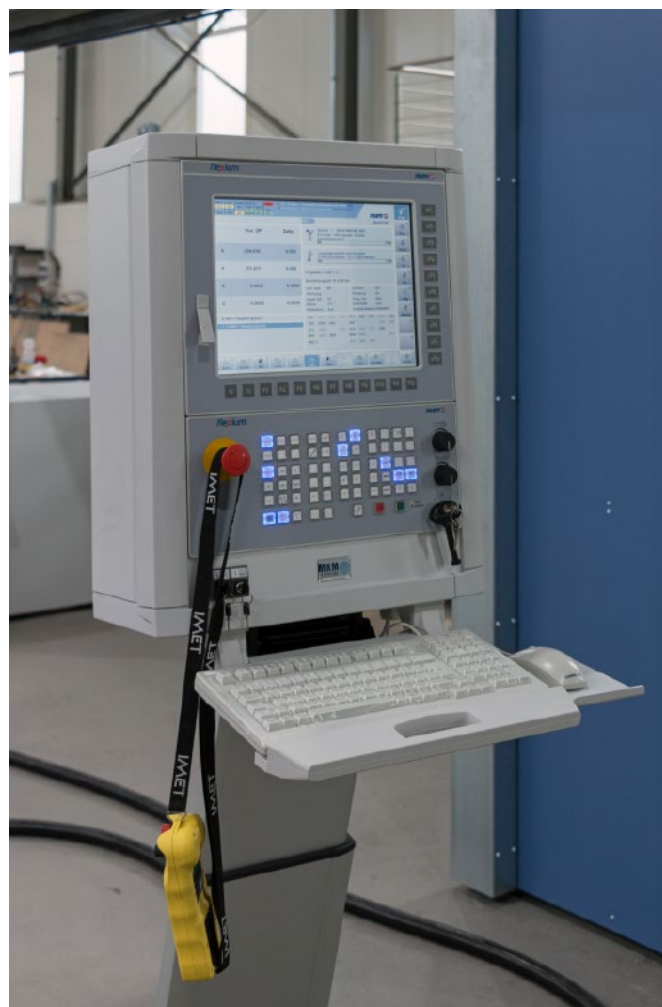
Flexium+ 68 control with a FS153i HMI and MP06 operating panel by NUM.
