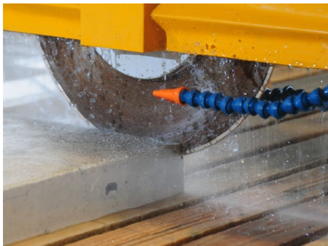
The saw blade cuts stone at up to 650 rpm and has a diameter of up to 1.3 m.
