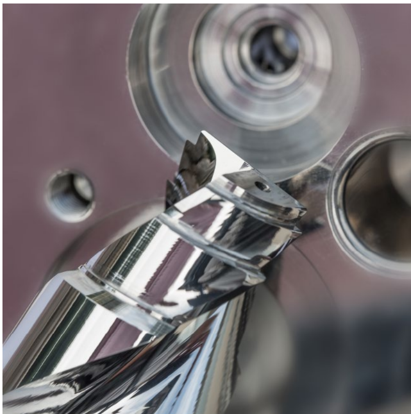
A special tool manufactured, polished and coated by HAM (step drill with several form steps) according to customer order.
