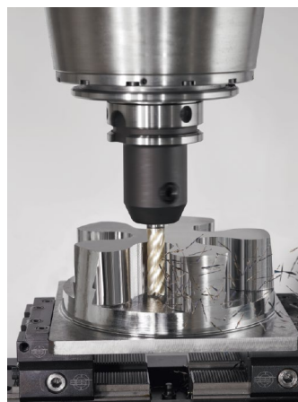
Solid carbide milling cutter MD133 Supreme from Walter Prototyp in use
