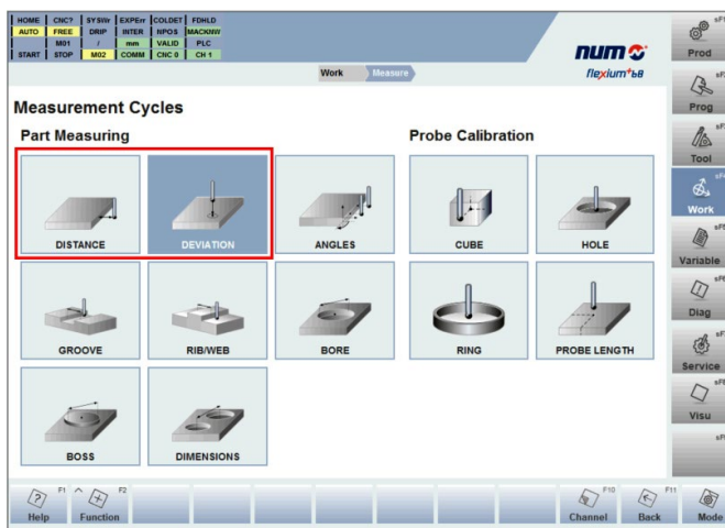
NUM's new software wizard enables CNC machine tool operators to easily handle probe measurements of parts and tools
