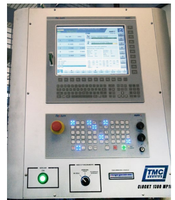
Control panel with NUM's Flexium + 68 CNC installed on the Tank 1300 MCM machining center.
