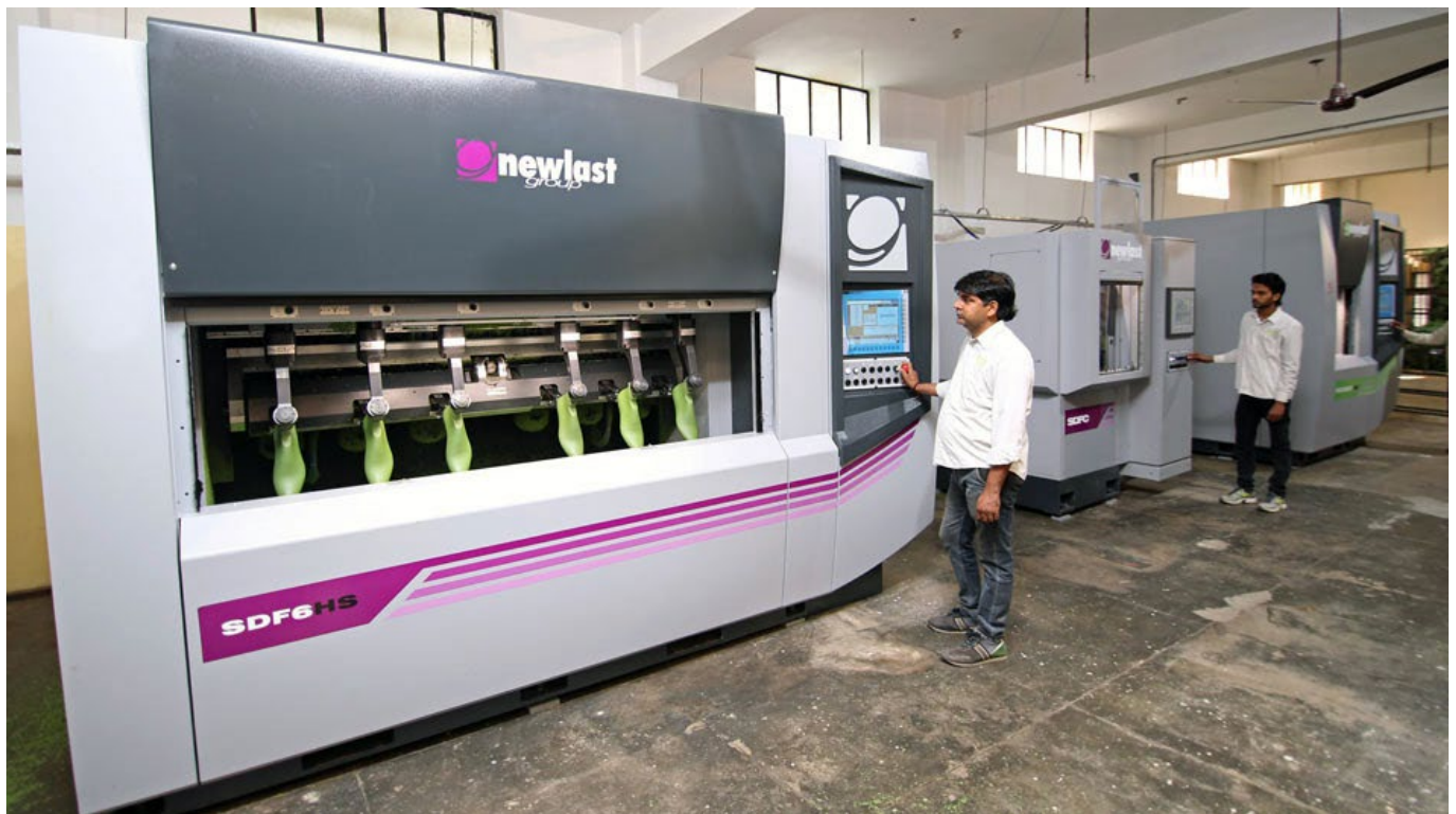
Rupmaya makes extensive use of Newlast CNC machine tools, which are based on NUM's Flexium CNC platform
