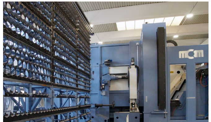
The Tank 2600's magazine is designed to accommodate 1,200 tools.
