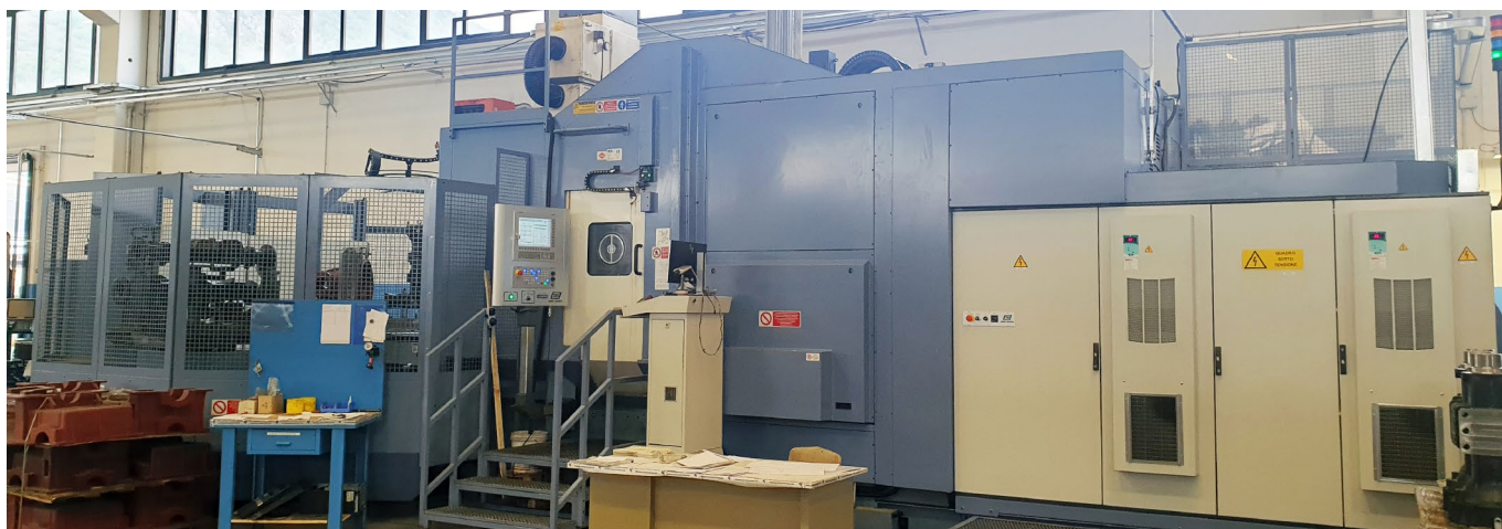
Tank 1300 MCM 4 axis machining center, 10 pallets and 400 tool magazine
