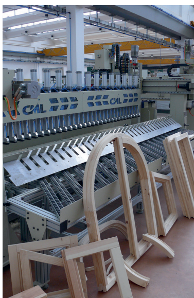
Machine with 64 axes for the production of window frames
