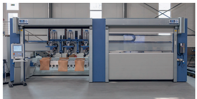
Innovative 17-axis milling machine for chair seats
