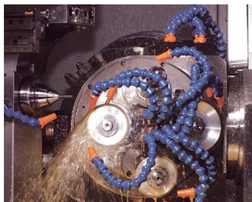
Mounted on a turntable, the wheel spindles can be equipped with 3 grinding wheels each. Associated with the 4-axis work-holding device, this multi-wheel spindle can perform a cylindrical grinding operation with no tool change.
