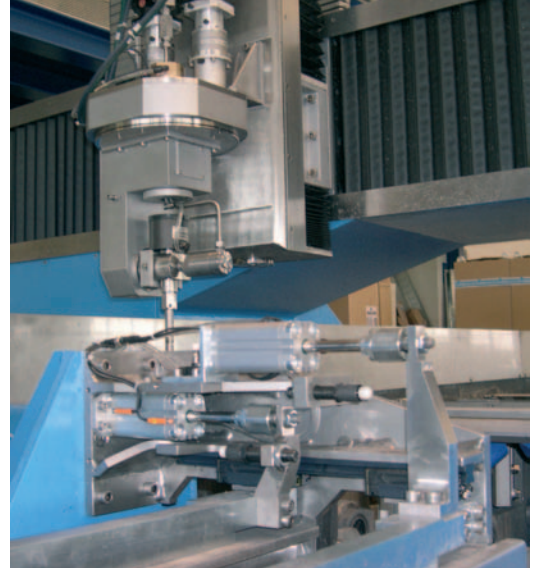
3D water jet cutting station, developed for Metzeler, a German automobile equipment supplier
