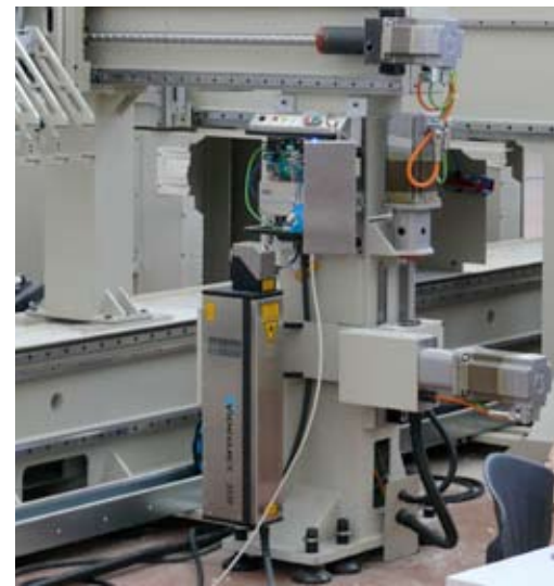
Laser device for different code printing (DATA-MATRIX, BAR CODE, TEXT CODE, etc.)
