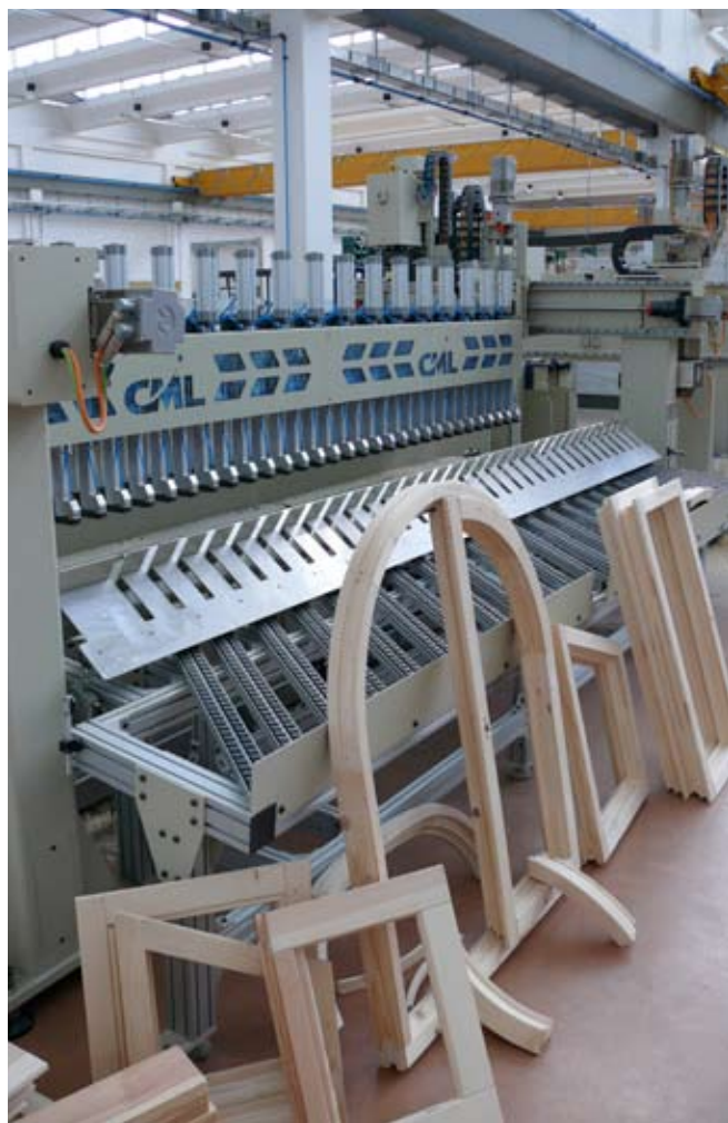
HELIOS machine with some examples of produced windows
