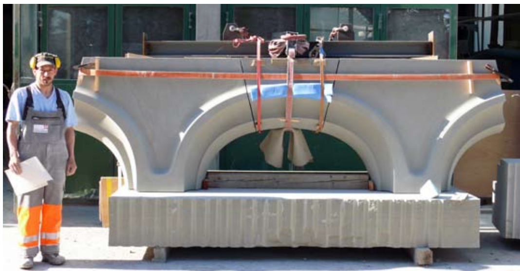
Complete machined arcade arches
