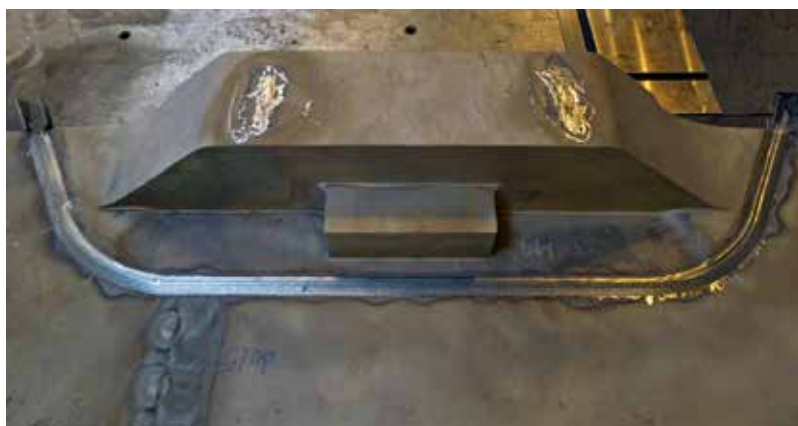
High-quality welded seams can be produced on steel and cast components using the SA system
