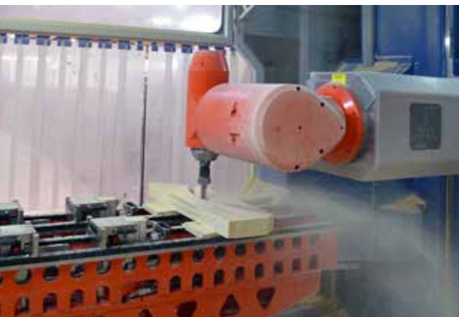
Top: twin-axis milling head in saw machining process
