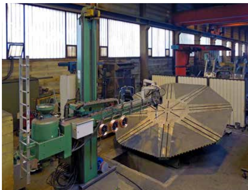
Left: welder operating the submerged-arc welding system using the joystick Right: submerged-arc welding system with rotary tilting table
