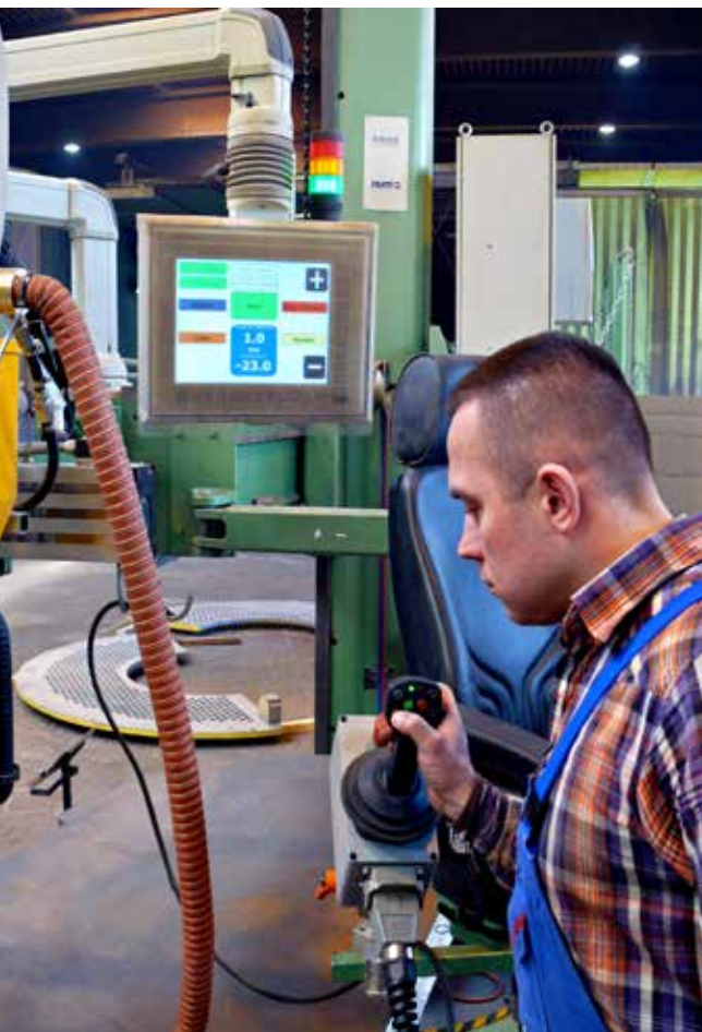
Bottom: worker setting up the system for the welding process using the joystick
