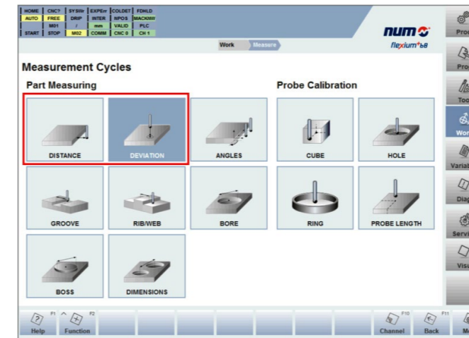
NUM's new software wizard enables CNC machine tool operators to easily handle probe measurements of parts and tools
