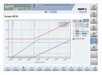
All these features are easily programmed with a single G function and a few parameters. For example, "Z100 G777 Q1 X40 P24 I25" tells the control to move the Z axes to the position Z100 mm, when 40 mm have been travelled the PLC output bit 24 will be set, and when the PLC input bit 25 is set then the execution of the next block will start, even before the Z axis has arrived at it's final position.
