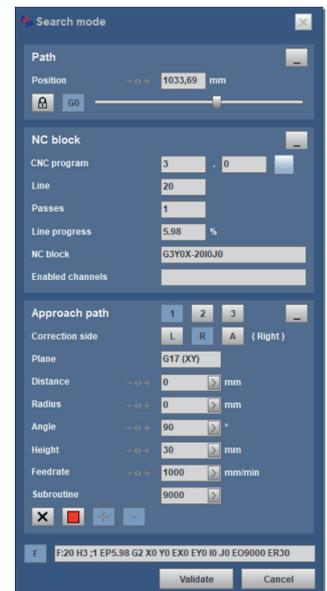
To use graphical supported SEARCH Mode on FlexiumPro systems the HMI option Flexium 3D Online-simulation (FPSW282155) is required.
