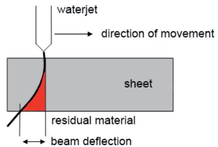
To ensure that no material is left behind, the standard feed behavior must be adjusted. The transitions between different feeds are defined as jumps. However, they are smoothed and executed with the maximum defined acceleration.
