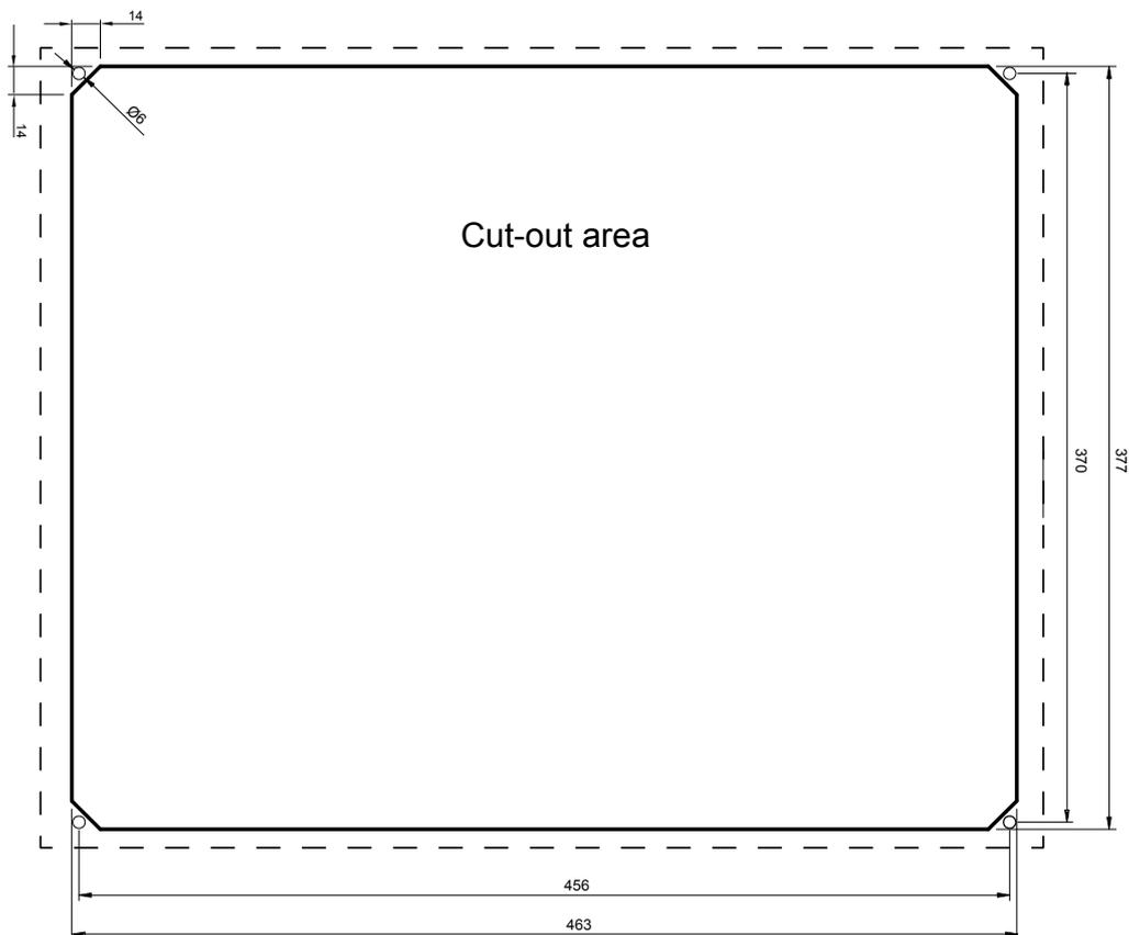
Cut-out in case of using back side mounting plate.
