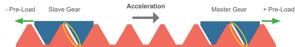
During strong acceleration phases, the needed thrust is higher than the pre-load: both motors/gears are thrusting in the same direction. The rack (red) moves. The pinion gears (in blue) are in motion.
