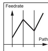
With linear feed variation, the transitions between different feeds are defined as straight lines.
