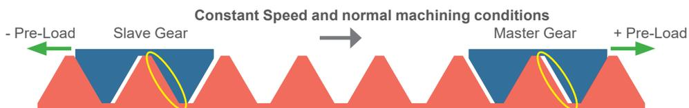
At constant speed, standstill and during machining, the pre-load compensates the backlash. The master position is the reference one. The rack (red) moves. The pinion gears (in blue) are in motion.
