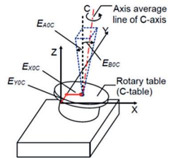
After measurement of the rotary axis imperfections, the errors will be entered in a table of data with the help of a worksheet macro. The error compensation is performed after defining a model of the machine structure which is considered as a succession of elements. Considering this model and based on the above values of errors, VECComp Rotary will calculate in real time the compensation to apply in order to position the Tool Center Point with the maximum accuracy.
