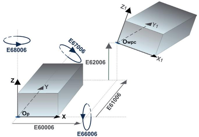
Owpc origin position shifts and Euler angles orienting the balanced coordinate system
