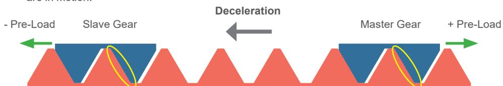
During strong deceleration phases the master gear recovers the backlash and retains the load. The rack (red) moves. The pinion gears (in blue) are in motion.
