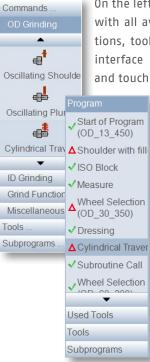
On the left-hand side is the "command tree" with all available functions (general definitions, tool selection, cycles, etc.). The user interface can work with mouse, keyboard and touch screen.
