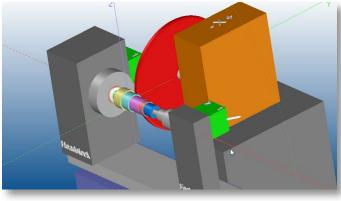
The Flexium 3D simulation tool has a Collision Detection Function.
