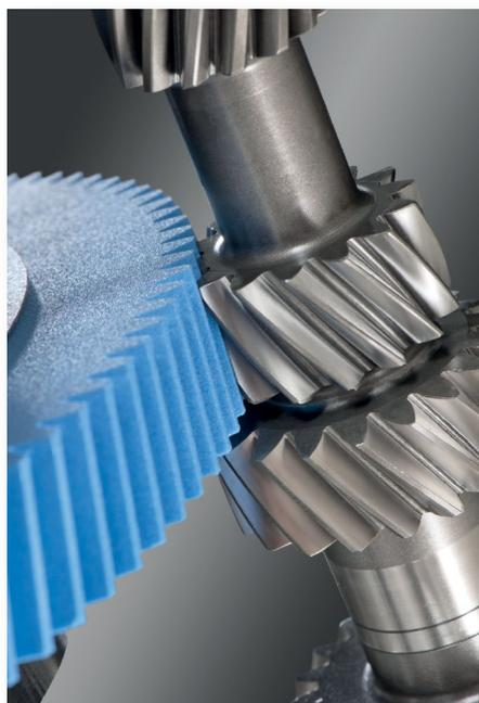
*Integration of a special electronic gear box (special axis / spindle synchronization) in the CNC system allowed to increase the speed of the honing wheel by more than 2.5.*
