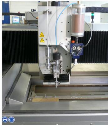
*By integrating special compensations and a corresponding mechanics, this machine is able to cut parts in the range of  $\pm 0.01$  mm by means of a water jet.*
