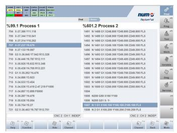
To increase the intelligibility of part programs the axis names can be indexed, e.g. X1, Y1, Z1, ... for channel 1, X2, Y2, Z2, ... for channel 2 a.s.o. On the one hand, the indexed axis names can be displayed in the user interface. On the other hand, they can also be used in the part programs.
