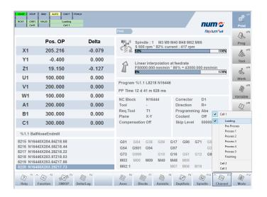
Regardless of the number of NCKs in the system, all information is displayed on a single HMI. Every station and every cell can be directly selected in any operating mode of the CNC system. The operator selects the corresponding function and does not have to bother about which axis channel and which CNC executes these functions. This provides an improved overview, increases operating speed and reduces inputting errors.
