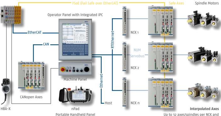
Up to 32 axes/spindles per NCK and more than 200 per CNC system
