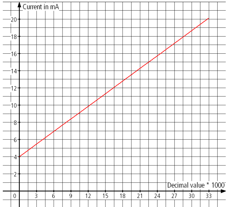
Figure 14: Representation of current values in relation to the decimal values in the coordinate system
