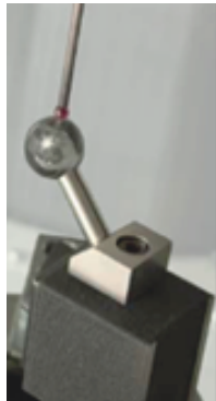
A calibration sphere, clamped on the work-piece table, is used as a reference feature for measurements
