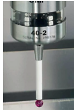
A calibrated 3D touch probe mounted in spindle
