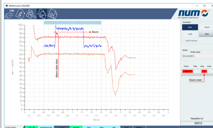
Fig. 36 MONITORING - with trace exceeding Alarm Amplitude limit, Alarm state.
