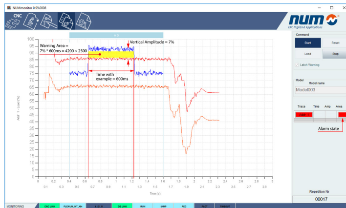
Fig. 41 MONITORING - with trace exceeding Warning Area limit, Alarm state.
