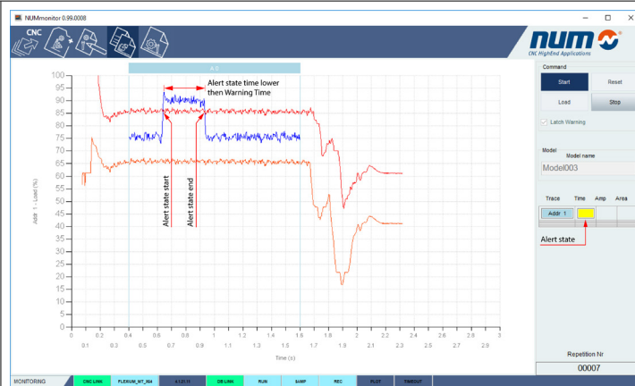
Fig. 32 MONITORING - with trace exceeding Vertical +%, Alert state
