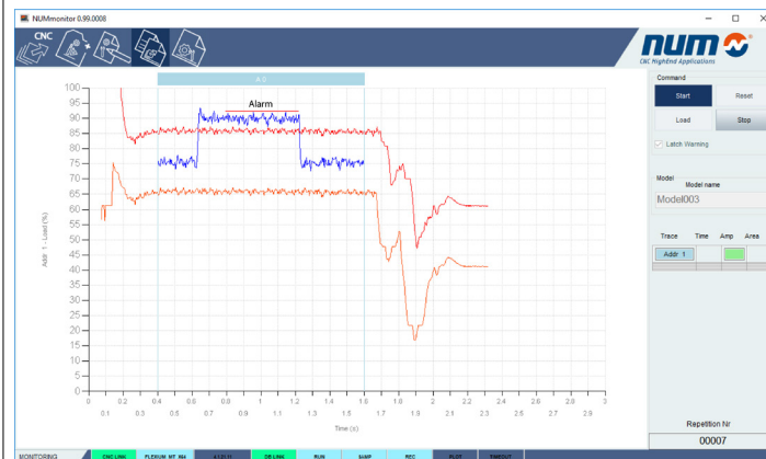
Fig. 35 MONITORING - with trace within Alarm Amplitude limit
