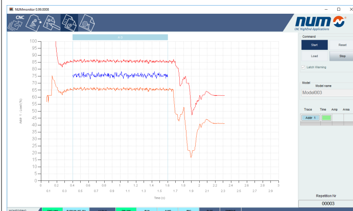
Fig. 31 MONITORING - with trace within Acceptance Area
