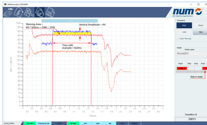
Fig. 40 MONITORING - with trace exceeding Warning Area limit, Alarm state.
