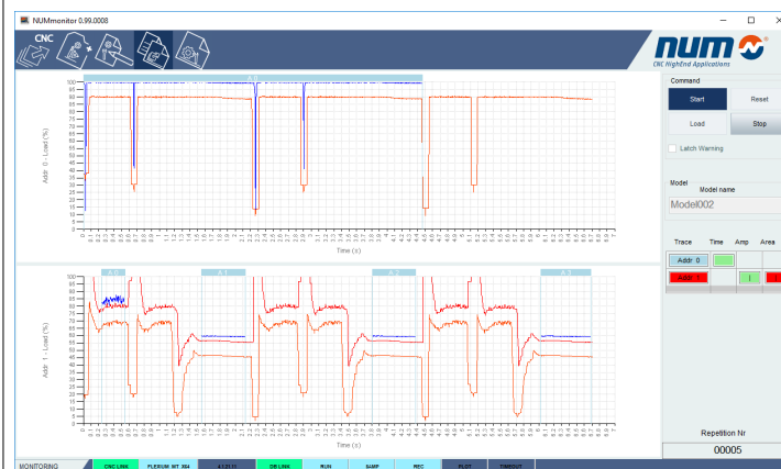
Fig. 43 MONITORING - Trace Addr1, Warning Amplitude Limit not in alarm state OR Warning Area Limit in alarm state (Trace in alarm)
