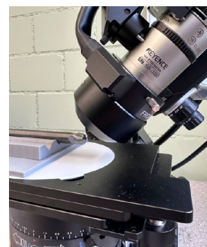
Measurement of the cutting edge on the full radius cutter at 45°
