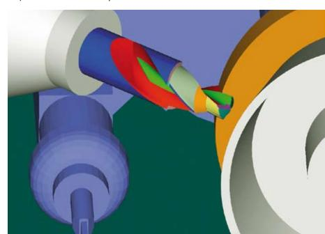
is very useful for monitoring the grinding position and cooling as well as for assessing the disc contact.
