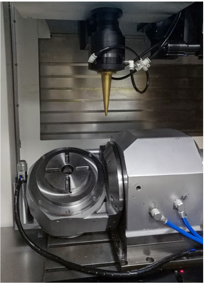
The ML125 machining centre has a dual laser head capable of both high speed and high quality cutting.
