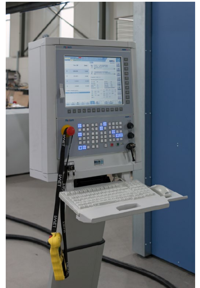
Flexium + 68 control with a FS153i HMI and MPO6 operating panel by NUM.
