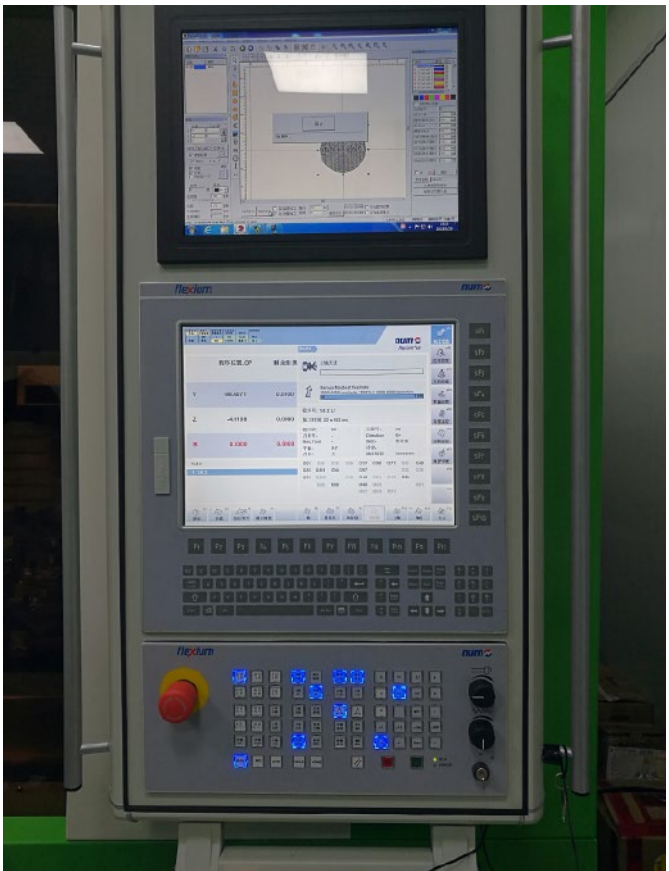
The HMI of the ML125 machining centre is based on NUM's Flexium touch screen technology.
