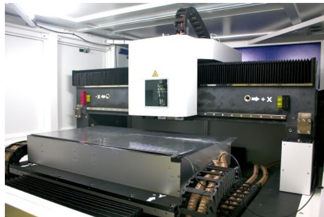
The gap between the laser cutting head and the workpiece is controlled very accurately, using a unique 'Dynamic Operator' function in NUM's Flexium software.
