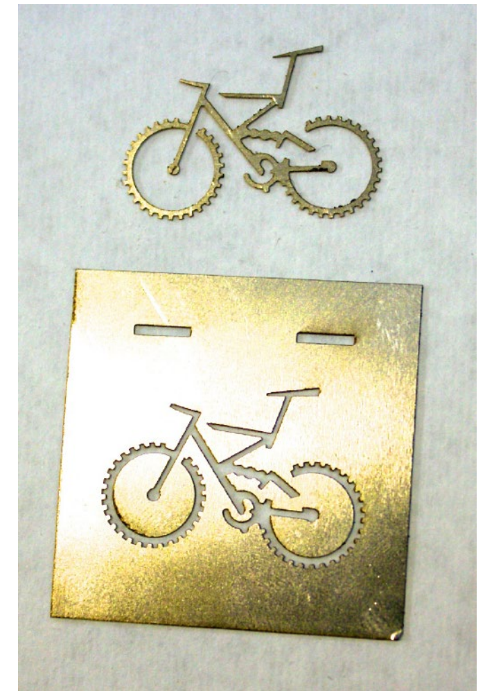
Legend Laser's new SRC-610 system can cut complex sheet metal parts to +/- 10 microns accuracy.
