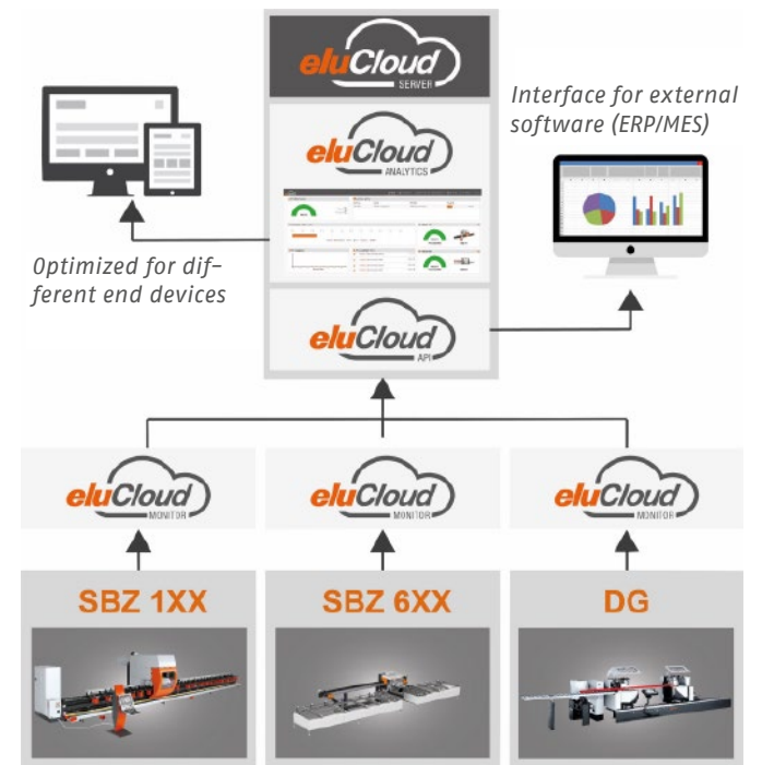
eluCloud: Machine data acquisition for versatile, personalizable data analysis.
