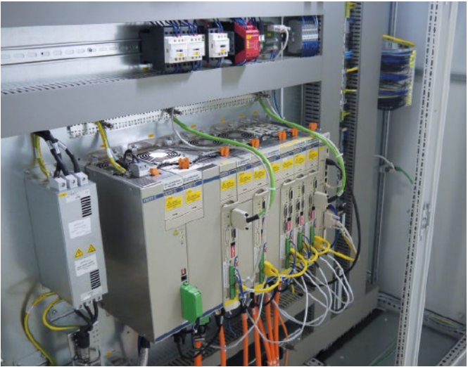
Detailed view of control cabinet: Flexium+ 68 CNC system with NUMDrive X with integrated safety solution.
