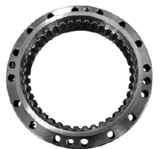
An internal gear after profile grinding.
