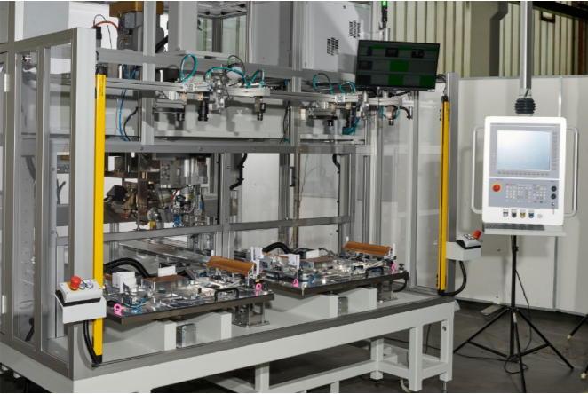
Hot stamping machine with a Flexium+ 68 control system. Two slide-in tables incl. 8 cameras for quality monitoring
