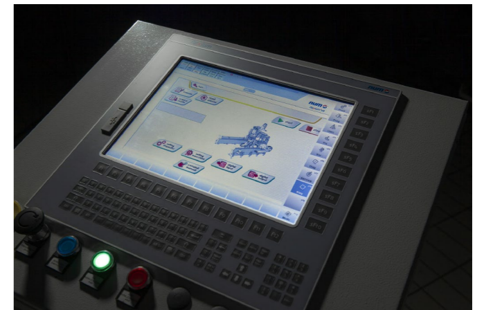
The system supplied by NUM is a Flexium+ 68, complete with digital drives from the MDLUX range, brushless motors in the single cable version and equipped with absolute encoders
