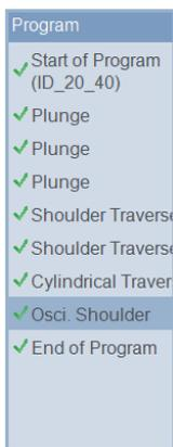
Select the grinding process at which the program is to continue again.
