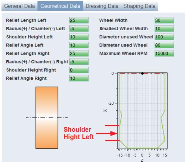
The shoulder height is added directly after the corner radius / chamfer. The total relief length does not change, only the section with the relief angle becomes shorter.
